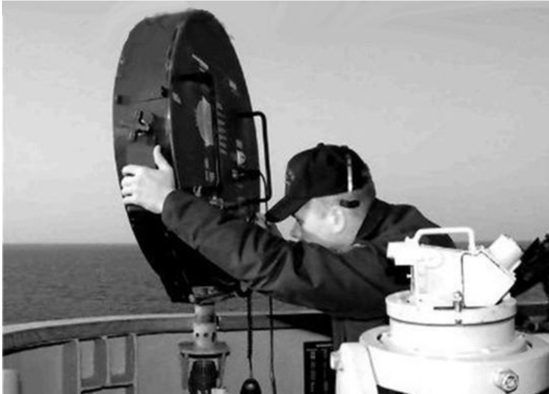
Long range acoustical device, developed by the Navy
